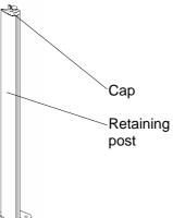
**Retaining post with ground sleeve:** anchor the sleeve plumb vertically in concrete, push the sectioning into the sleeve and then slide the retaining post on. Clamp the post in place with the hexagonal SW13 screw.
