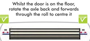
The Axel will protrude 11" (280mm) beyond the drum wheel at each side
