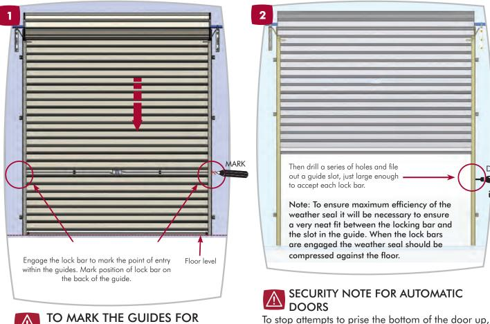
TO MARK THE GUIDES FOR THE LOCK BAR HOLES, THE DOOR MUST BE FULLY CLOSED
