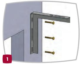
Fix the brackets in place at each side of the opening.
