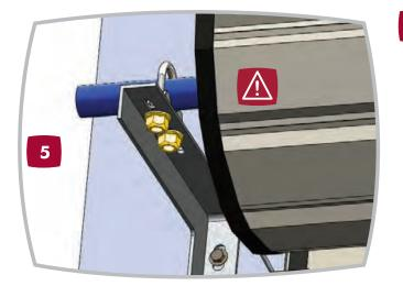
5 Tighten the 'U' bolts with the bottom rail at the start position as shown in point 2.
