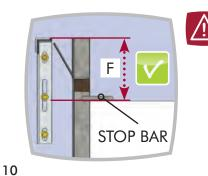
For automatic installations the measurement from the top of the horizontal leg of the support bracket to the bottom edge of the stop bar is critical. It must never be less than:
