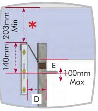
D=35mm Minimum on doors with 30mm guides D=60mm Minimum on doors with 50mm guides
