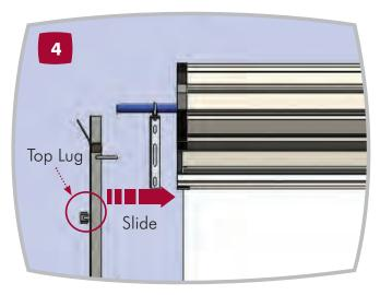
Drill wall and fix the top lug of 5 each guide with a 10mm x 65mm sleeve anchor or coach screw.
