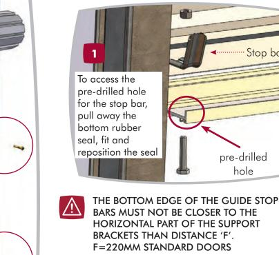
BARS MUST NOT BE CLOSER TO THE HORIZONTAL PART OF THE SUPPORT F=140MM MINI DOORS IF THIS IS NOT OBSERVED THE DOOR WILL **BE DIFFICULT TO CLOSE**
