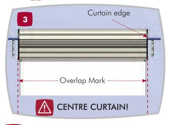
ENSURE THE DOOR CURTAIN IS CENTRED. IF ADJUSTMENT IS REQUIRED, CENTRE THE DOOR ROLL BY LIFTING THE CURTAIN AND AXLE TOGETHER
