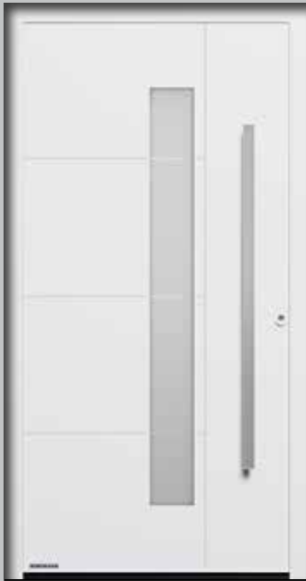
Style 877 Stainless steel handle HOE 610, matt float design glass with 3 clear stripes, triple thermal insulation glass, U_D -value up to approx. 0.9 \text{ W}/(\text{m}^2\cdot\text{K})^*
