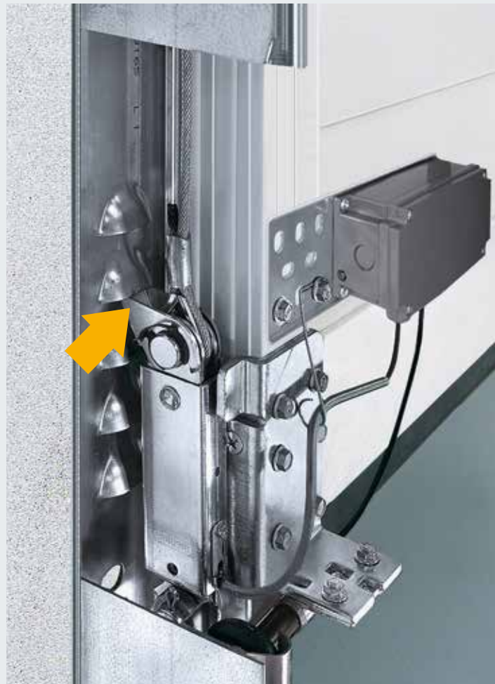
The locking hook of the arrestor kit automatically latches if the door is forced upwards.
