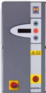
AK 500 FUE-1 FU control in plastic housing, IP 54, three-phase, 400 V
