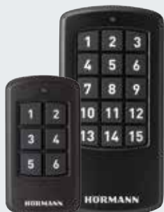
Industrial hand transmitter HSI 6 BS, HSI 15 BS // NEW To control up to 6 doors (HSI 6 BS) or 15 doors (HSI 15 BS), with extra-large buttons for easier operation with work gloves, impact-resistant housing Protection category: IP 65
