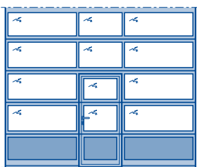
Sectional door ALR F42 with wicket door with trip-free threshold
