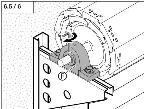
• Tighten the screws on the bearing (F).
