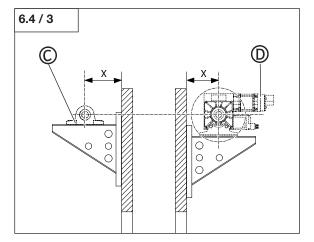
6.4/4 • Set up the distance to the wall (X) on both sides. 6.4 / 5
