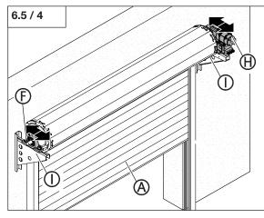
• Position the door curtain (A) between the guide rails (E).
