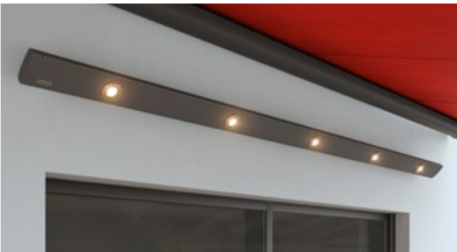
markilux LED Spotline The elegant light bar in a powder-coated aluminium housing, that can be fitted almost anywhere. The LED Spots can be tilted and swivelled. Available in two sizes: 180 cm with 3 spotlights and 300 cm with 5 spotlights.
