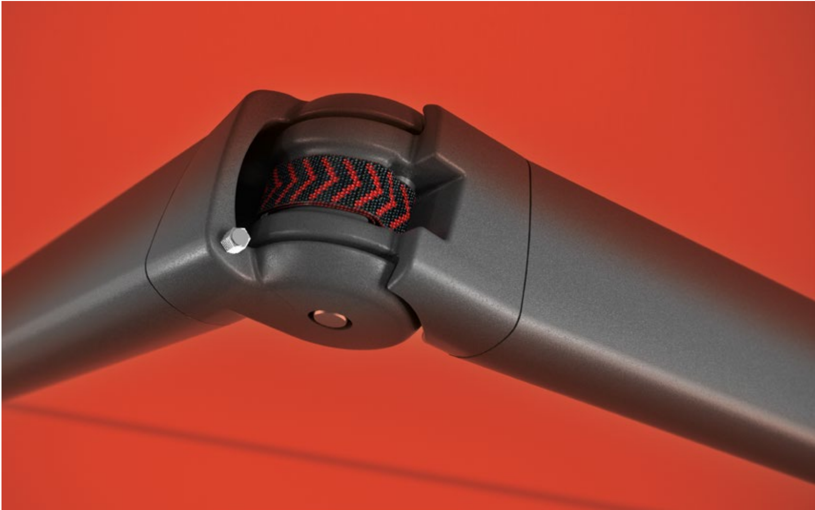
Bionic tendon markilux developed the bionic tendon from high-tech fibres, and used nature as its inspiration to create optimum power transference as well as friction-free and virtually noiseless folding of the arms. The safety and durability of the arms also impressed when it achieved more than 50,000 arm flexions in independent tests.
