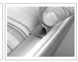
2. This is pushed into the upper piping groove and is engaged by swiveling.
