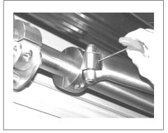
5. Secure the eccentric bolt with the threaded pin. Check the new setting of the articulated arms by retraction and extension of the awning.
