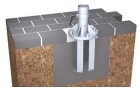
**Dowel-anchored plate** galvanized, weight approx. 25 kg.  $a = 25 \text{ cm}, x = \square 50 \text{ cm}, t = 1.2 \text{ cm}, z = \emptyset 1.8 \text{ cm}$
