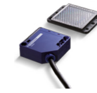
Extra 628 reflection light opto sensor • 24-240 V AC, 12-240 V DC, IP 54 • Range: 5 m • Can only be used as a pulse generator
