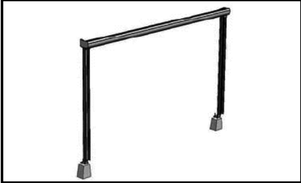
Picture 11, Put the supports with the gutter in an upright position
