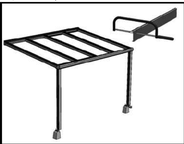
Picture 17, place support beams / saw last 2 cover profiles
