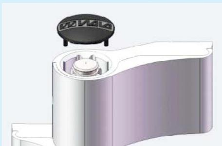
2. Open the door, remove the M4 screw (3mm allen key).
