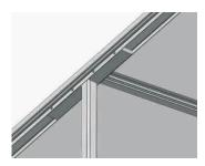
Image shows gutter channel fitted.
