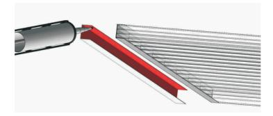
The capping can then be knocked onto the sheet using a white rubber mallet.
