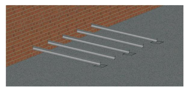
IMPORTANT: Use Roofing Square to ensure the bar used is held square to the wall.
