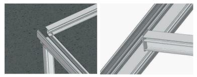
Starting with the End Glazing Bar, push this bar into the wall plate so that it is pushed back as far as possible and ensure the outside profile lines up with the edge of the wall plate. Rest the other end of the glazing bar on the radius inner section of the gutter section.
