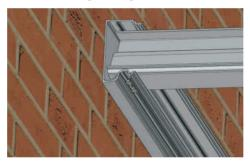
Make sure the glazing bar is in line with the gutter beam, then using the same fixing method as the wall plate secure the glazing bar to the gutter section. Your pre drilled holes will determine where you drill through on the radius of the gutter section. Please see diagram below:
