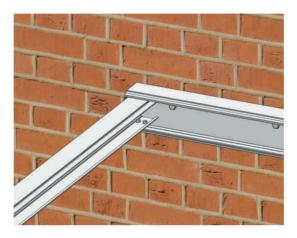
Using suitable wall fixings, fix the wall plate to the wall.
