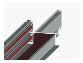
6. Once you have married the two beams together you must leave at least a <u>3mm gap</u> between the two but no greater than 5mm
