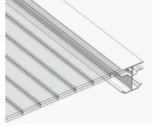
Place your next glazing bar into the polycarbonate sheet and push firmly into the channel. Please see diagram below. Fix the glazing bar onto the wall plate and gutter section, as previously described in step 8 make sure all glazing bars have a bead of sealer down both edges of the glazing bar to prevent water ingress as described above.
