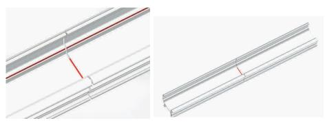
10. Apply a generous amount around the edges of the flat plates inside the gutter and ensure all gaps are filled with Sudaflex internally.
