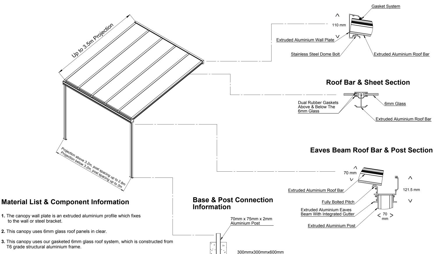
**4.** The frame of the canopy is made from 70mm x 75mm x 2mm aluminium box section.
