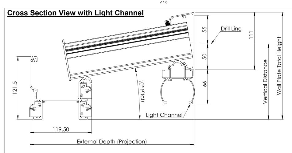
Example distance to appropriate drill hole on wall plate 10 degree roof pitch.
