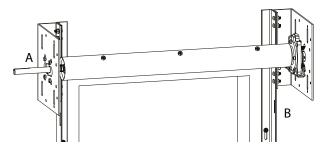
vi. Adjust the position of the axle, making sure it is centrally aligned within the end plates. The design is such that each end of the axle will align with the inside face of the end plate flap that is used to attach to the channel angles. This ensures that the curtain will roll up evenly on the axle, as there will be no end-lock overlap.
