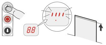
**Note:** The closed position should should be set at 4 o'clock. This is particularly important for <u>Single Skin</u> doors.
