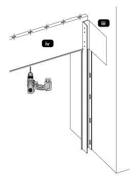
v. Flx the remaining main fixing angle to the other side of the structure, bolt on the second angle then fix the second end plate to the second angle.
