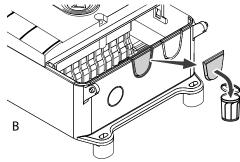
iii. Insert and connect connection cable in the open cable entry A (from below) or B (from above) and properly tighten cable glands.
