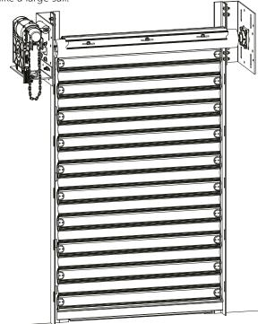
viii. Once the curtain has been fully installed, haul it up until the bottom lath is hanging about 100mm down from the underside of the end plates.
