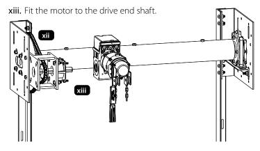
**xiv.** Secure the motor with the 4 bolts supplied in the 'Bearings' section of the fittings kit.
