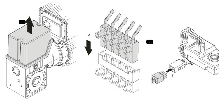
iii. Feed the cable to where the control unit is to be installed. Ensure the cable is secured along its length by using appropriate containment or clips.
