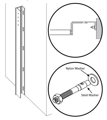
**iii.** Fix the end plate to the second angle with the M8 nuts and bolts.
