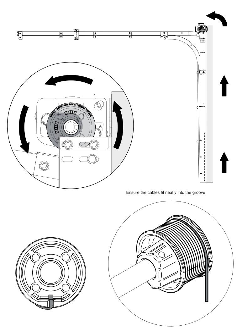
Check paperwork or spring tension label located on the spring for number of turns
