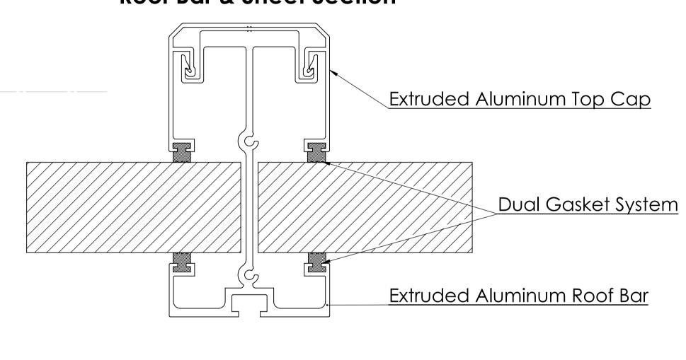
Wall Plate & Roof Bar Section
