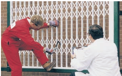
SeceuroGuard 1001 undergoing a simulated attack test
