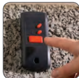
Garage control - light on, open - close and vacation lock.
