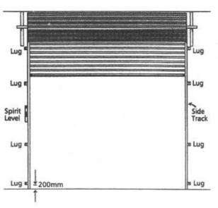
Slide the track on to the door curtain, allowing 4mm clearance. Hold the guide in position against the wall and mark the location of the top lug holding screw. USING A SPIRIT LEVEL TO ENSURE THAT THE SIDE TRACK IS ABSOLUTELY VERTICAL, fix the track in position by means of the adjustable lugs and 40mm coach screws ensuring that they are evenly spaced, with the bottom lug approximately 200mm from the floor.
