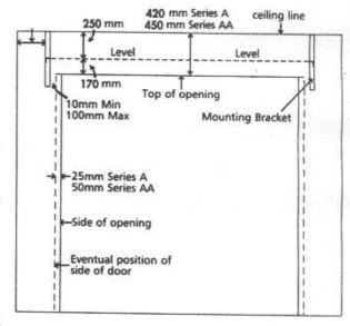
The second mounting bracket should then be positioned. The use of a line level or spirit level and straight edge is recommended as IT IS VITAL THAT THE BRACKETS ARE EXACTLY LEVEL WITH EACH OTHER, otherwise the door will not sit square. The minimum 250mm series A and 280mm series AA dimensions must be maintained. Automatic doors require the motor side bracket to be lowered by 5mm after brackets have been levelled off.
