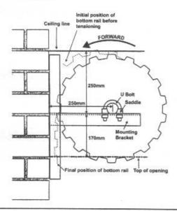
Tension should now be applied to the spring by rotating the door about 1½ times in a forward direction, as shown. The amount of tension required to give the best operation may vary with individual doors. Final adjustment should be made on completion of the job.
