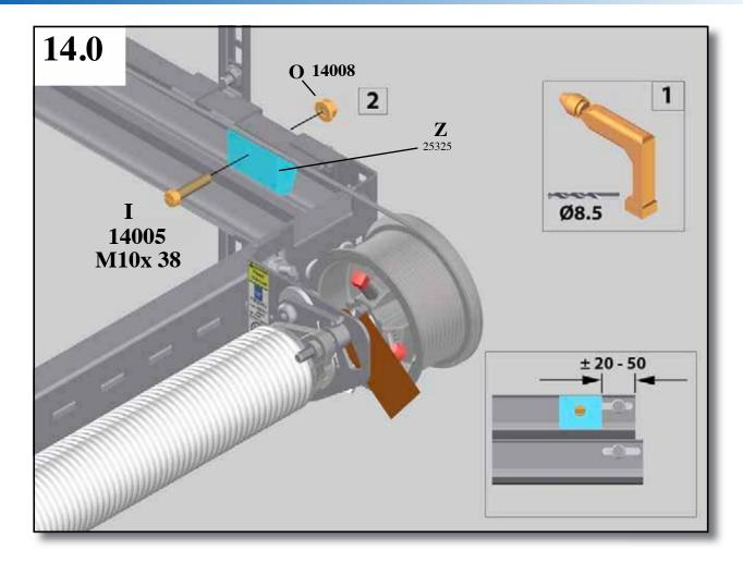
Rubber track stoppers to be fitted once door has been set to max opening point.
