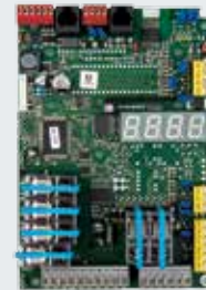
Extension PCB for controls: BK 150 FU E-1 (E FU H) AK 500 FUE-1 (E FU H)
