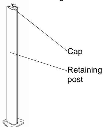
**Retaining post with ground sleeve:** anchor the sleeve plumb vertically in concrete, push the sectioning into the sleeve and then slide the retaining post on. Clamp the post in place with the hexagonal SW13 screw.
