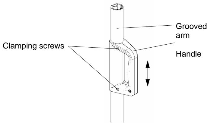
3.7 Set its height so that the awning is tensioned dead straight.
