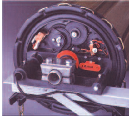
Detail A: End view of Drive Unit with access cover removed showing limit switches, cam gears and cut out switch. Also shown is the Manual emergency disconnect lever and the anchor block attached to wall bracket with dual anchor pins into the Drive Housing.
