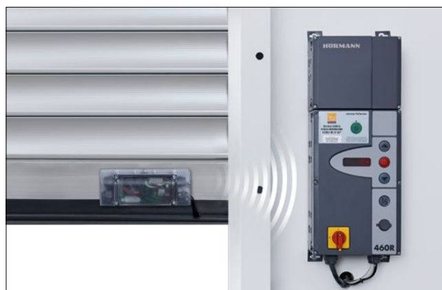
Optional: Radio transmission unit For transmission of signals from the door curtain to the control via Bluetooth – instead of a coiled cable. Power supply via a high-performance battery. For controls: 445 R / 460 R
