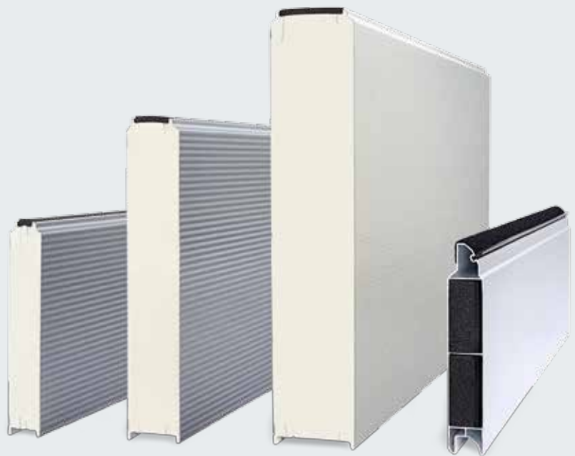
Double-skinned steel sandwich sections with thermal break in three thicknesses: 42, 67 and 100 mm, acoustic section
