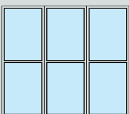
Prepared for site infill (max. 16 kg/m 2 ) resting within the frame Frame in terra brown (RAL 8028)
