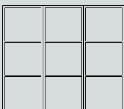
Smooth sheet steel infill Sheet thickness 1.5 mm
