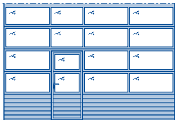
Sectional Door APU 67 Thermo with Wicket Door with Trip-Free Threshold
