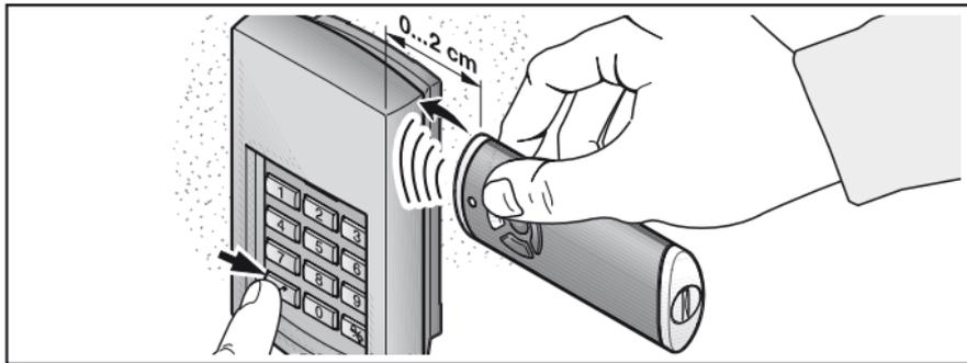
1. Hold the hand transmitter to the right of the radio code switch.
