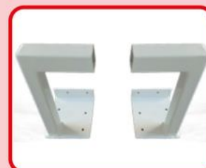
Window Saddles 58003 Left and Right bracket, to be used in conjunction with Installation Post 38 x 38. Bracket fixing options, horizontally into window frame, or vertically into reveal, or both.
