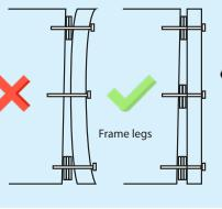
If packers have been used, ensure each fixing point has packers to prevent the frame distorting when tightening fixings.
