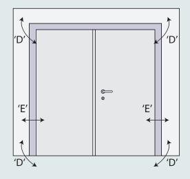
Open the door leaf, make the adjustments to the jacking bolts and close to check the door is hanging true.
