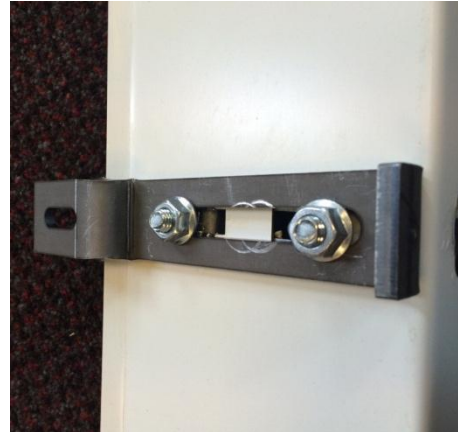
Fig 2 – Bracket ( SG199R0 ) with extended bolts attached
