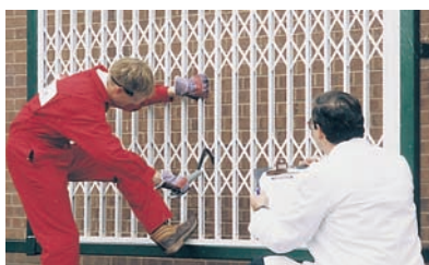
SeceuroGuard 1001 undergoing a simulated attack test
