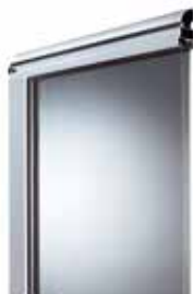
Frame profile with 19 mm synthetic double glazing, tinted green; light transmission of approx. 70%
