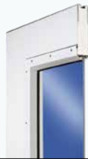
18 mm double glazing, 6 mm laminated safety glass or 21 mm ISO laminated safety glass, with steel glass retaining strips. New: Category 3 waterproof in heavy rain
