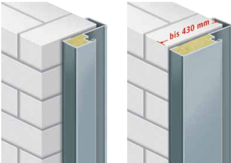
Mortar-free wall plug assembly
