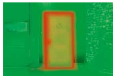
Visible energy loss without thermally separated door
