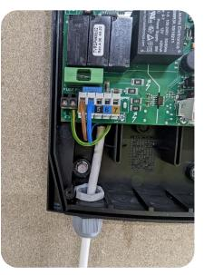
Wires are to be fed up through the bottom of the control board & secure using a panel plastic gland supplied with the control box.
