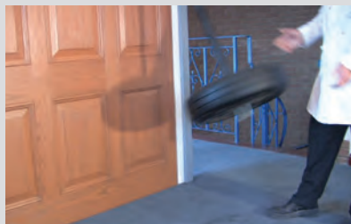
Impact tested for strength
