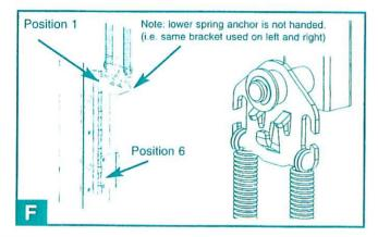
Still with the door in the open position and wearing eye protection fit lower spring anchors as shown and fit springs to spring anchors in orientation shown (See fig F).
