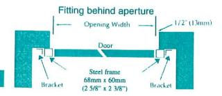
**Dimensions of steel frames are:** 136mm (5 3/8") greater than opening width, 68mm (2 11/16" greater than opening height, 60mm (2 3/8") deep all round.
